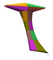
Autogyro Calidus Rotor Mast Cover, 3D model
