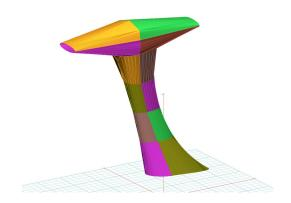
Autogyro Calidus Rotor Mast Cover, 3D model
