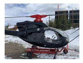
Rotorway Exec 162 Rotor Mast Cover
