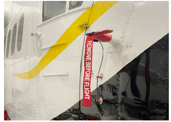
DeHavilland DH-6 Pitot Cover with Static Port Plugs
