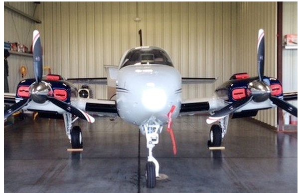
Beech Baron 58 Engine Inlet Plugs, Cowl Top Plugs, Heater Inlet, Pitot Cover
