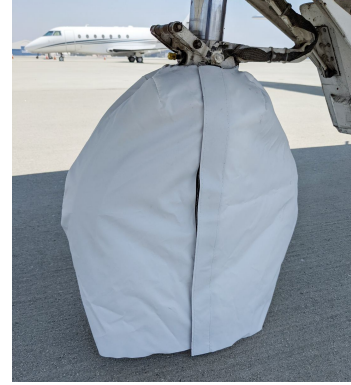
CJ1 Nose Gear Tire Cover, test fit
