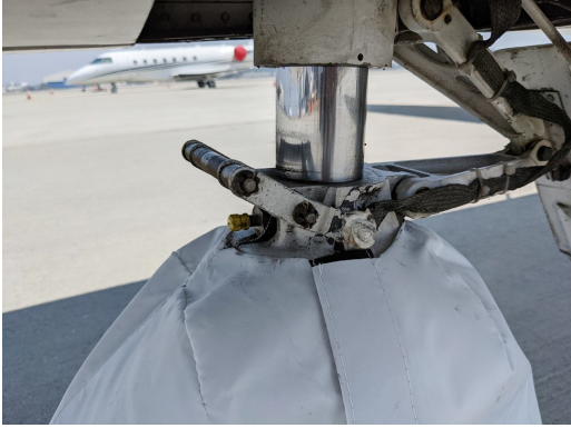
CJ1 Nose Gear Tire Cover, test fit
