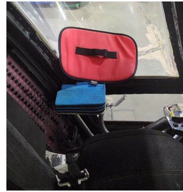
Boeing Vertol CH-47 Logger Window Plug
