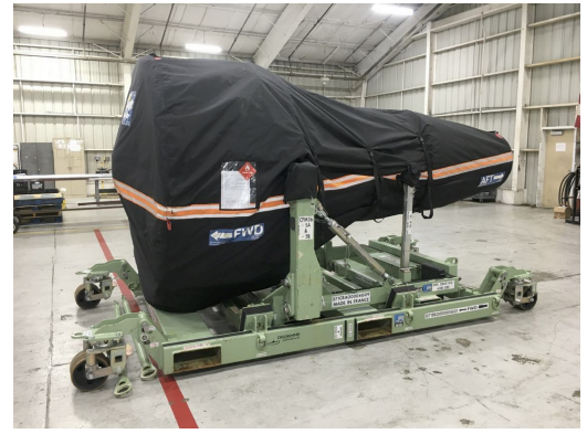
CFM56-5B Off Link Cover, fully enclosed
