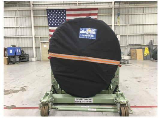
CFM56-5B Off Link Cover, fully enclosed
