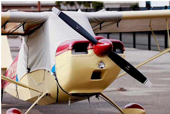
Bellanca Citabria Over-the-Top Canopy Cover, extended to cover gas caps
