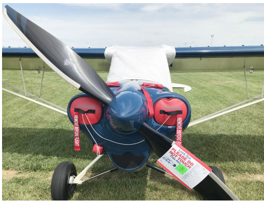
Cub Crafters EX2 Canopy Cover, Engine Plugs
