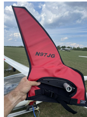
Schempp-Hirth Ventus-2B winglet/wingtip pads
