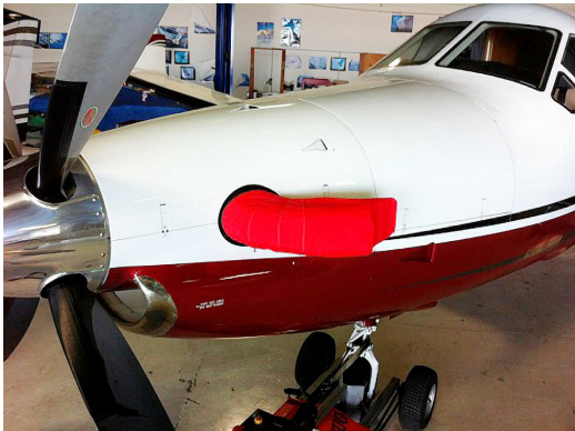
King Air C90 Insulated Engine Cover, 3D model Pilatus PC-12 Exhaust Cover, Fully Enclosed, for protection against corrosion.
