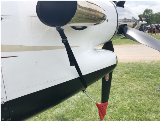
Beech C90A Prop Tie-Down
