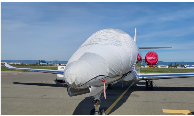
Cessna Citation Latitude (680A) Cockpit/Nose Cover, Doesn't Cover Pitot Tubes
