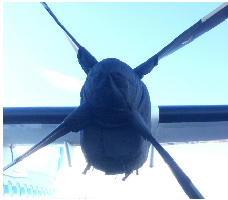
ATR-72-202 Insulated Engine & Prop Hub Covers
