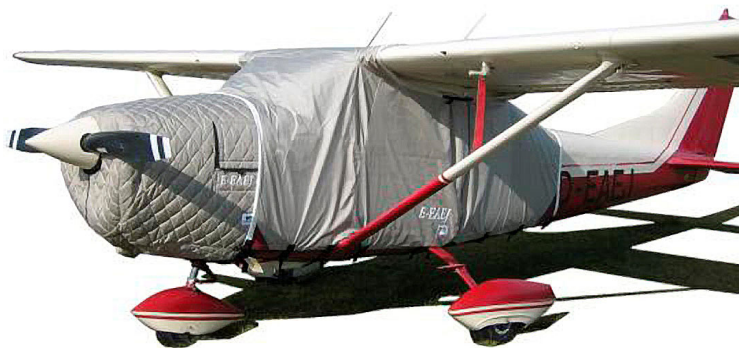
Cessna 182 Insulated Engine Cover ext. to l.e of nose gear, Extended Canopy Cover Insulated Hangar Blanket on Cessna 182
