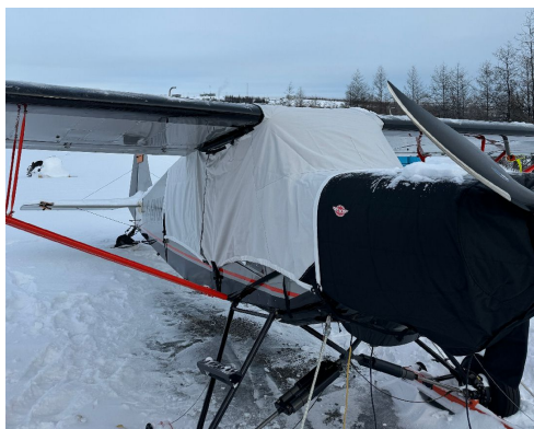
Bushmaster Canopy & Insulated Engine Covers
