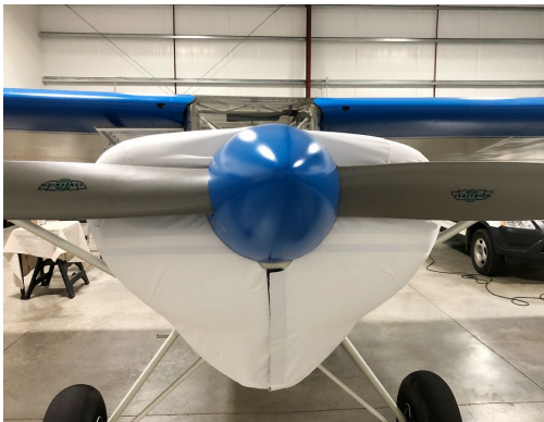
Bearhawk Patrol Engine Cover, test fit cover
