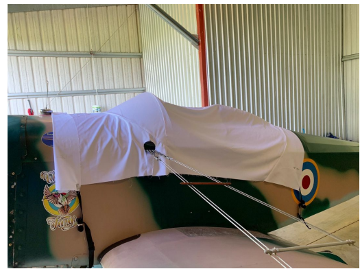
Bowers Flybaby Canopy Cover, test fit design
