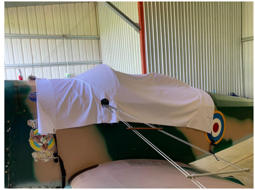
Bowers Flybaby Canopy Cover, test fit design
