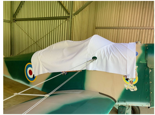
Bowers Flybaby Canopy Cover, test fit design
