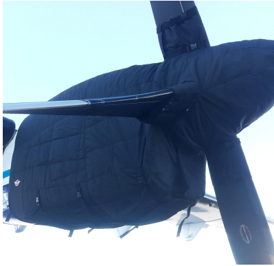
ATR-72-202 Insulated Engine & Prop Hub Covers
