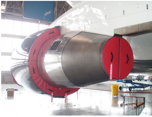
Airbus A330 Intake Plug, framed bi-fold type Exhaust Plugs Ship Set, incl. Fan Thrust Reverser and Exhaust Plugs P/N: B767-200
