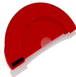
Airbus A330 Intake Plug, framed bi-fold type
