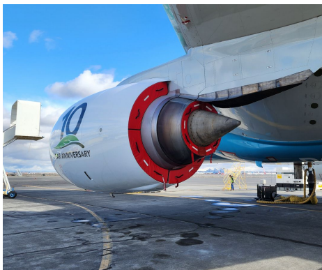
Boeing 777 Bypass Plugs & Turbine Exhaust Plugs, RR Trent 800 Engines
