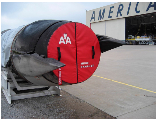
MD80 JT8D Exhaust Plug, Folding Type
