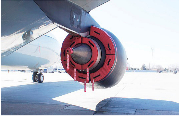
RC-135W Bypass Vent and Exhaust Plugs
