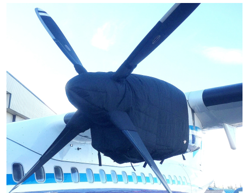
ATR-72-202 Insulated Engine & Prop Hub Covers
