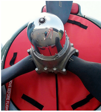
C-46 Radial Engine Intake Plug
