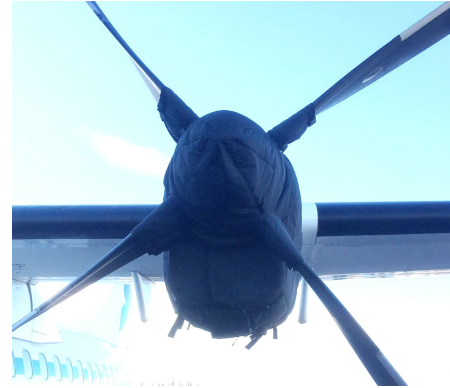
ATR-72-202 Insulated Engine & Prop Hub Covers
