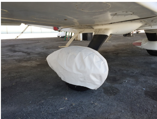
Grumman AA5 Main Wheelpant Cover, test fit
