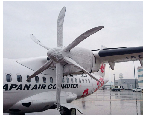
ATR-42/72 Engine Cover, 6-Blade Prop/Spinner Cover
