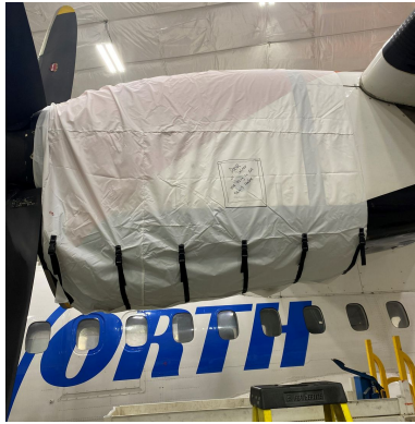
ATR-42/72 Engine Covers, test fit cover
