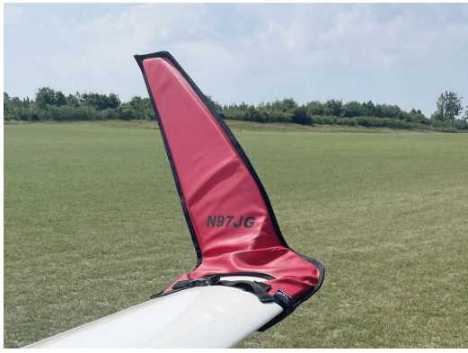
Schempp-Hirth Ventus-2B winglet/wingtip pads
