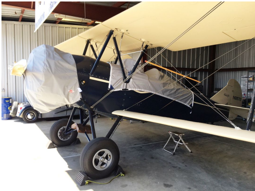
Wacon Cabin Biplane ZQC-6 Insulated Engine Cover Travel Air 4000 Canopy and Engine Covers, light weight travel type
