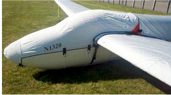
Schweizer SGS 1-26B Canopy/Nose, Wings & Empennage Covers
