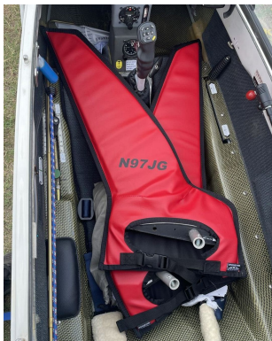
Schempp-Hirth Ventus-2B winglet/wingtip pads
