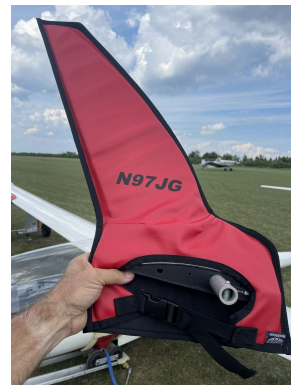
Schempp-Hirth Ventus-2B winglet/wingtip pads
