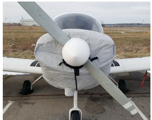
Alarus CH-2000 Insulated Engine Cover
