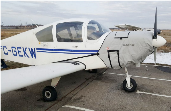
Alarus CH-2000 Insulated Engine Cover
