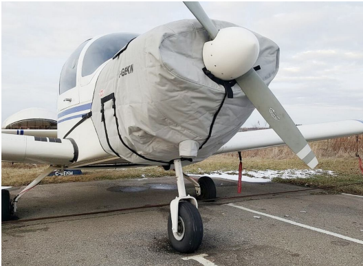
Alarus CH-2000 Insulated Engine Cover
