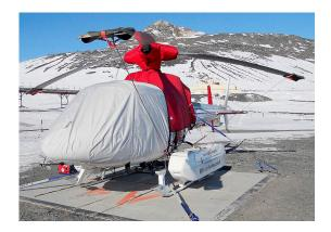
AS350 Windshield Cover, pinches in door AS350 Bubble Cover w/ Cargo Mirror, Blade Tie-downs, Insulated Engine, Insulated Main Rotor Hub and Insulated Tail Rotor Covers
