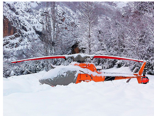
AS350 Bubble Cover, Insulated Main & Tail Rotor Covers, Blade Covers with tid-down detail
