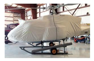
AS350 Windshield Cover, pinches in door jambs AS350 B3 Main Body Cover (Covers Bubble/Cabin, Engine Area and Exhaust)
