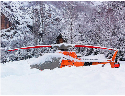
AS350 Bubble Cover, Insulated Main & Tail Rotor Covers, Blade Covers with tid-down detail
