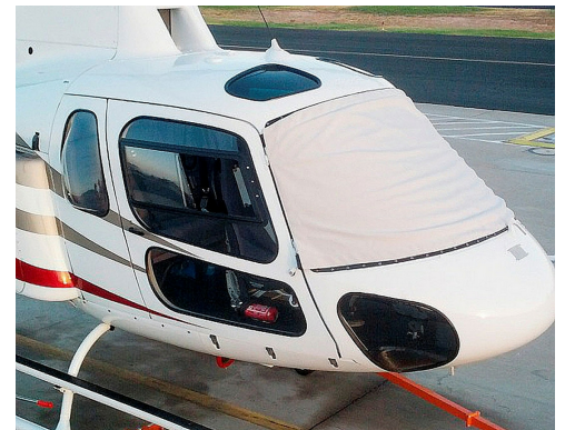
AS350 Windshield Cover, pinches in door jambs
