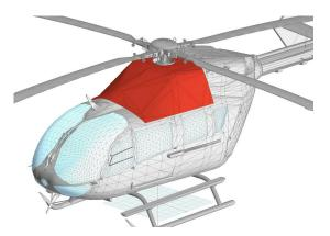
Barrier Inlet Filter Cover, 3D Rendering
