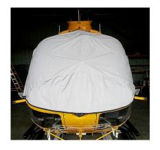
Eurocopter EC-145 Main Body Cover, also covers the bottom belly EC-135 Windshield/Skylights Cover, pinches in door jambs
