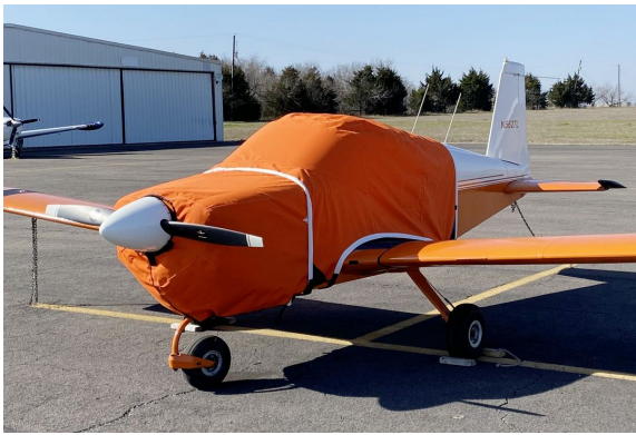
AA-1 Extended Canopy & Fully Enclosed Engine Cover
