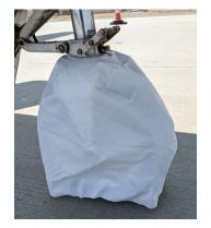
CJ1 Nose Gear Tire Cover, test fit
