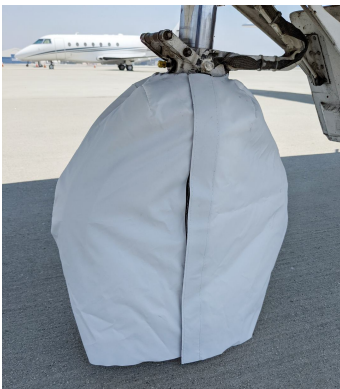
CJ1 Nose Gear Tire Cover, test fit
