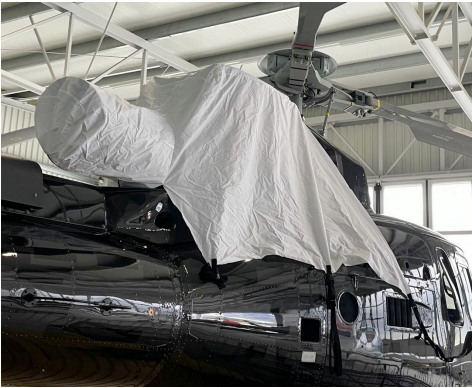
AS350 Intake/Exhaust Cover, test fit cover
