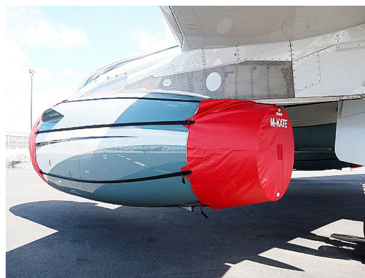
Airbus A319 Intake/Exhaust Covers set, IAE V2500
