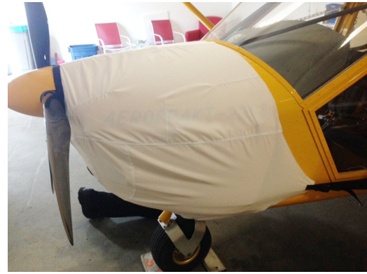
A-22 Engine Cover, test fit
