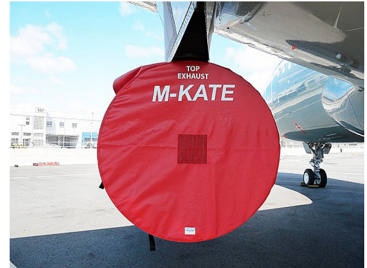
Airbus A319 Intake/Exhaust Covers set, IAE V2500
