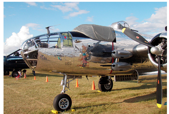
Mitchell B25 Cockpit Cover (Snap-On Type)
