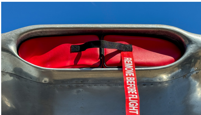
Douglas A26 Invader Oil Cooler Inlet Plugs
