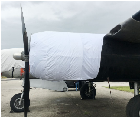
Douglas A-26 Engine Cover, test fit cover
