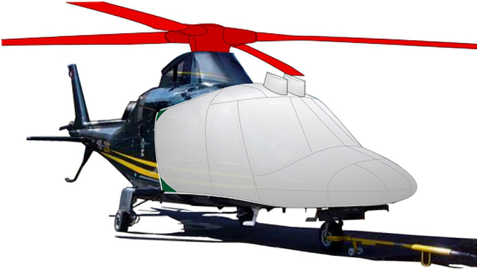
Agusta Leonardo A169 Bubble Cover with Wire Strike, 3D model Agusta 109 Bubble, Rotor Hub & Blade Covers (illustration)
