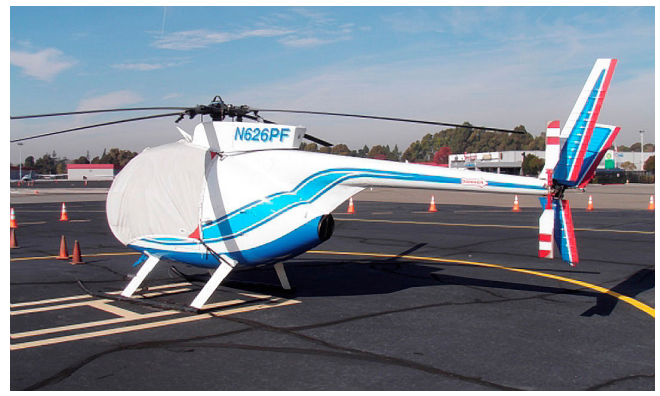
MD500C Bubble Cover with Wire Strike detail
