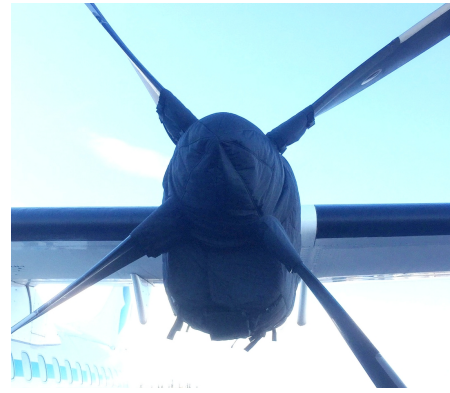
ATR-72-202 Insulated Engine & Prop Hub Covers
