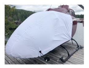
Bell 505 Bubble Cover, test fit cover
