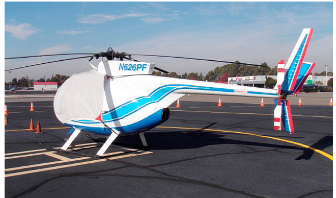
MD500C Bubble Cover with Wire Strike detail
