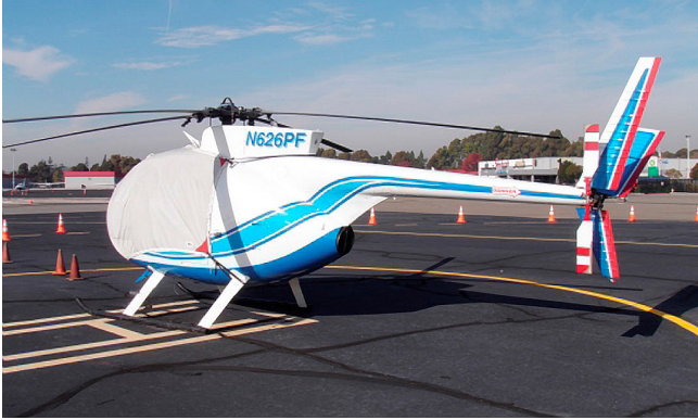
MD500C Bubble Cover with Wire Strike detail
