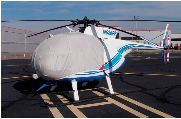
MD500C Bubble Cover with Wire Strike detail
