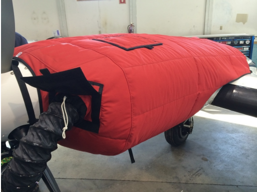
Cessna 402 Insulated Engine Cover with Heater
