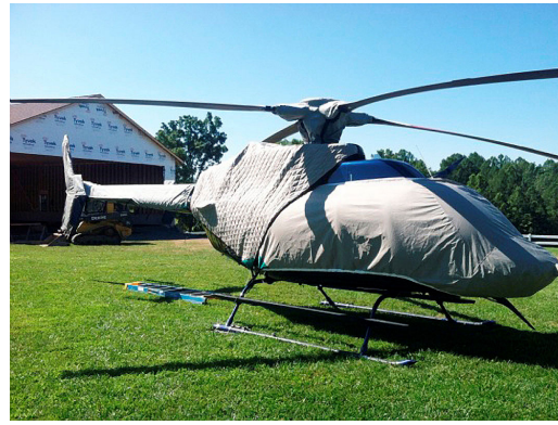
Bell 407 Covers: Bubble, Insulated Engine, Rotor Mast, Blades, Tailboom, Vertical Stabilizer and Tail Rotor
