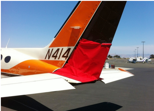
Cessna 414 Rudder Openings Cover (bird barrier)
