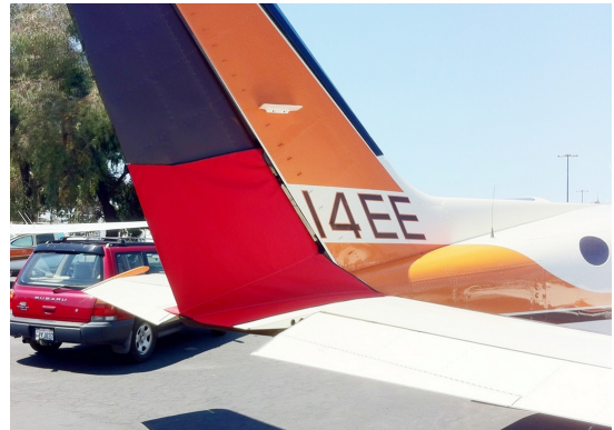
Cessna 414 Rudder Openings Cover (bird barrier)
