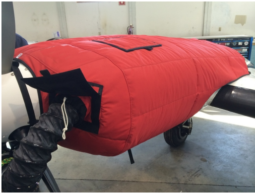
Cessna 402 Insulated Engine Cover with Heater
