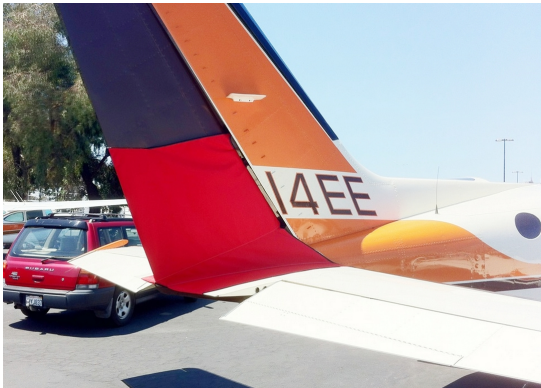
Cessna 414 Rudder Openings Cover (bird barrier)
