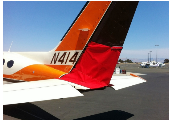
Cessna 414 Rudder Openings Cover (bird barrier)
