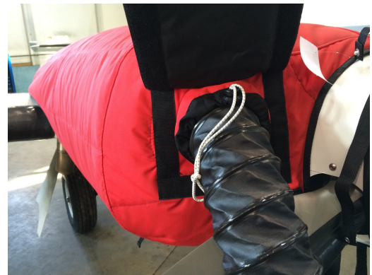
Cessna 402 Insulated Engine Cover with Heater
